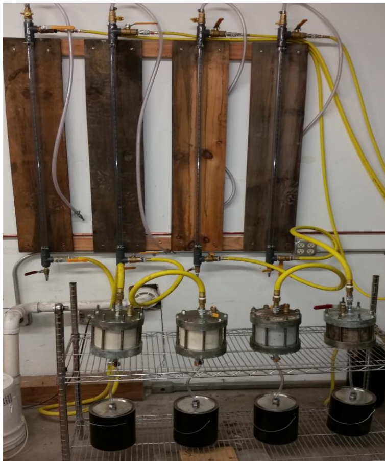
Photo #2 – CRD C-48 Testing Set-up
