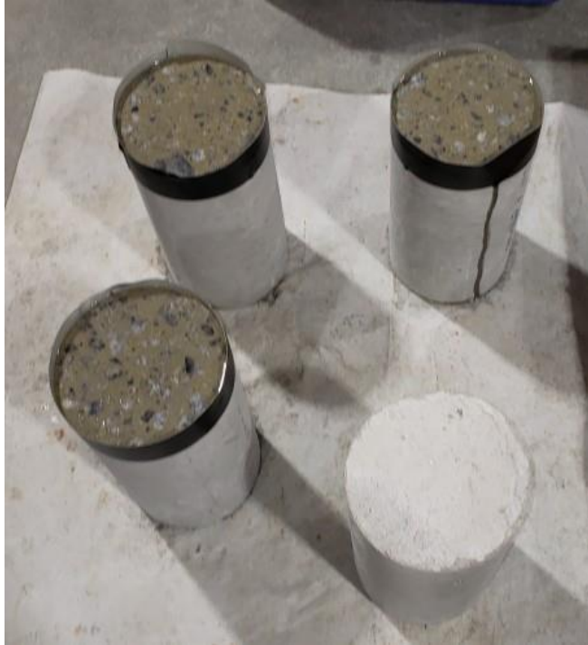
Photo #1 – Cylinder Specimens with Vetrofluid Freshly Applied
