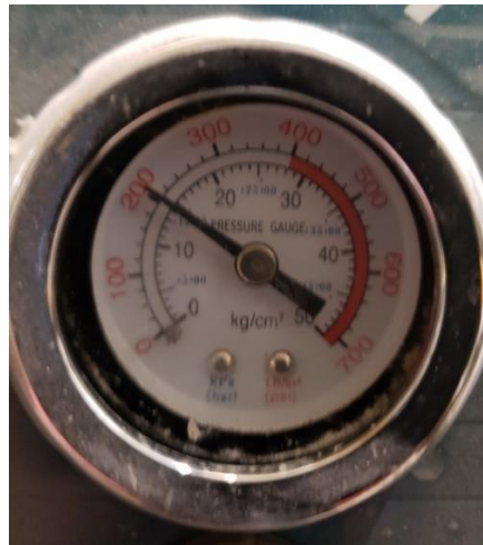
Photo #3 – Pressure Gauge Showing Applied Pressure
